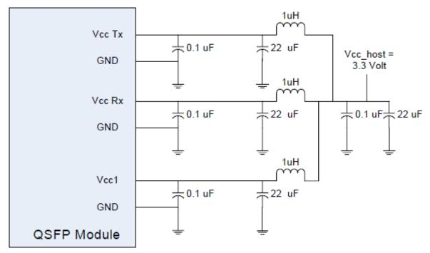
**Recommended Host Board Power Supply Filtering**
