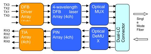
Figure 1: 40Gb/s QSFP IR4 Transceiver Block Diagram
