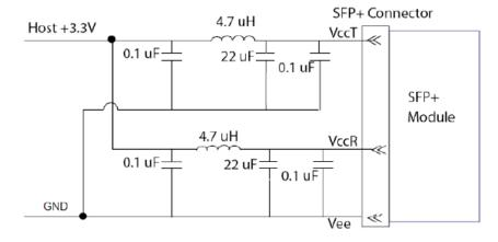
**Recommended Host Board Power Supply Circuit**
