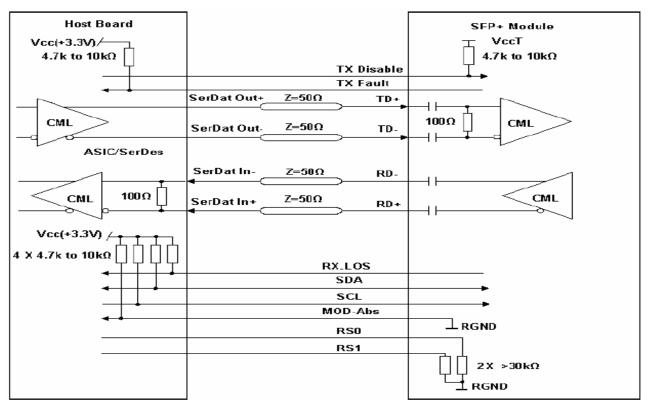
**Recommended High-speed Interface Circuit**
